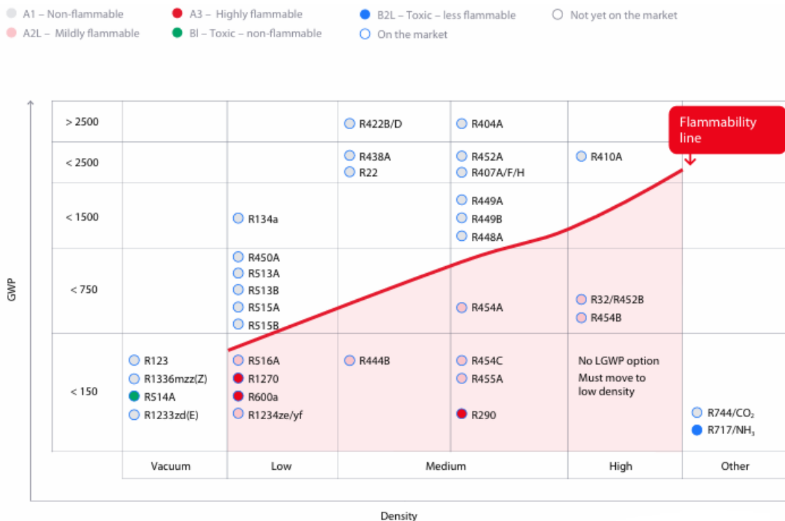
Figure 7. Carbon -chain-based Refrigerants (HCs, HFCs, HFOs, HCFCs), GWP versus density (pressure) of the main refrigerant groups [7].
